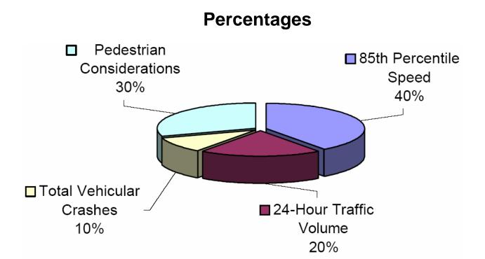
Speed differential ranks heaviest in the consideration for installing traffic calming devices, followed by pedestrian generators, minimum daily traffic volume and total vehicular crashes. Point accumulation will be determined from the chart below. A total of 20 points is possible.
