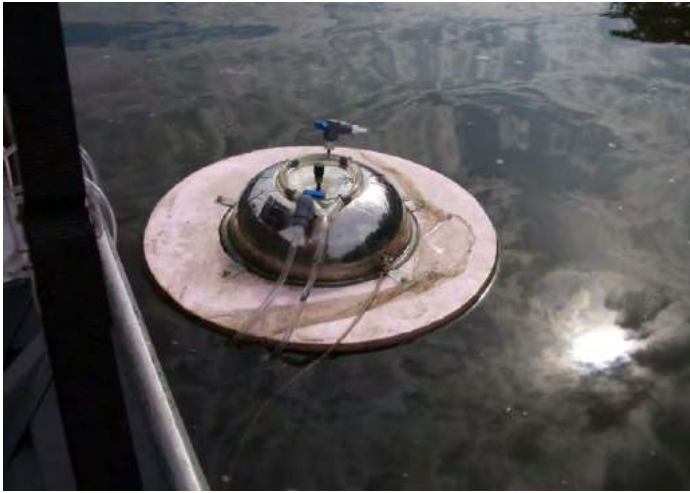
Figure 4. Floating Dome Reaeration Measurement Device (Credit: Koenig)
