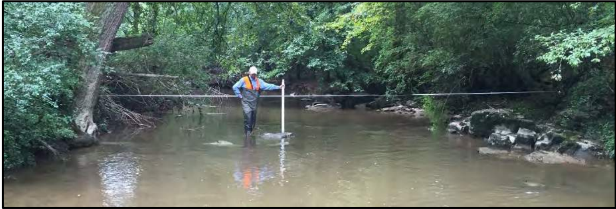
Figure 8. Example of Cross-section Field Measurements
