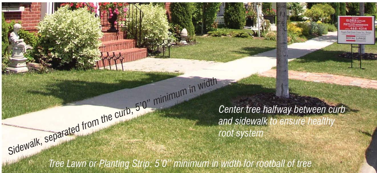
Streetscape Detail: Detached 5'-0" sidewalk located 5'-0" from the back of curb with planting strip and shade tree. KEEP IT SIMPLE!!!
