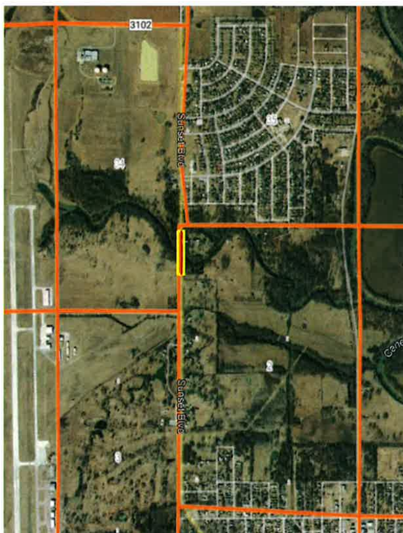
Section Geometry: The approximate centerline of survey is along the Osage/Washington County Lines, which is also a correction meridian. The correction meridian creates atypical section geometry and positioning, as shown in the above exhibit.
