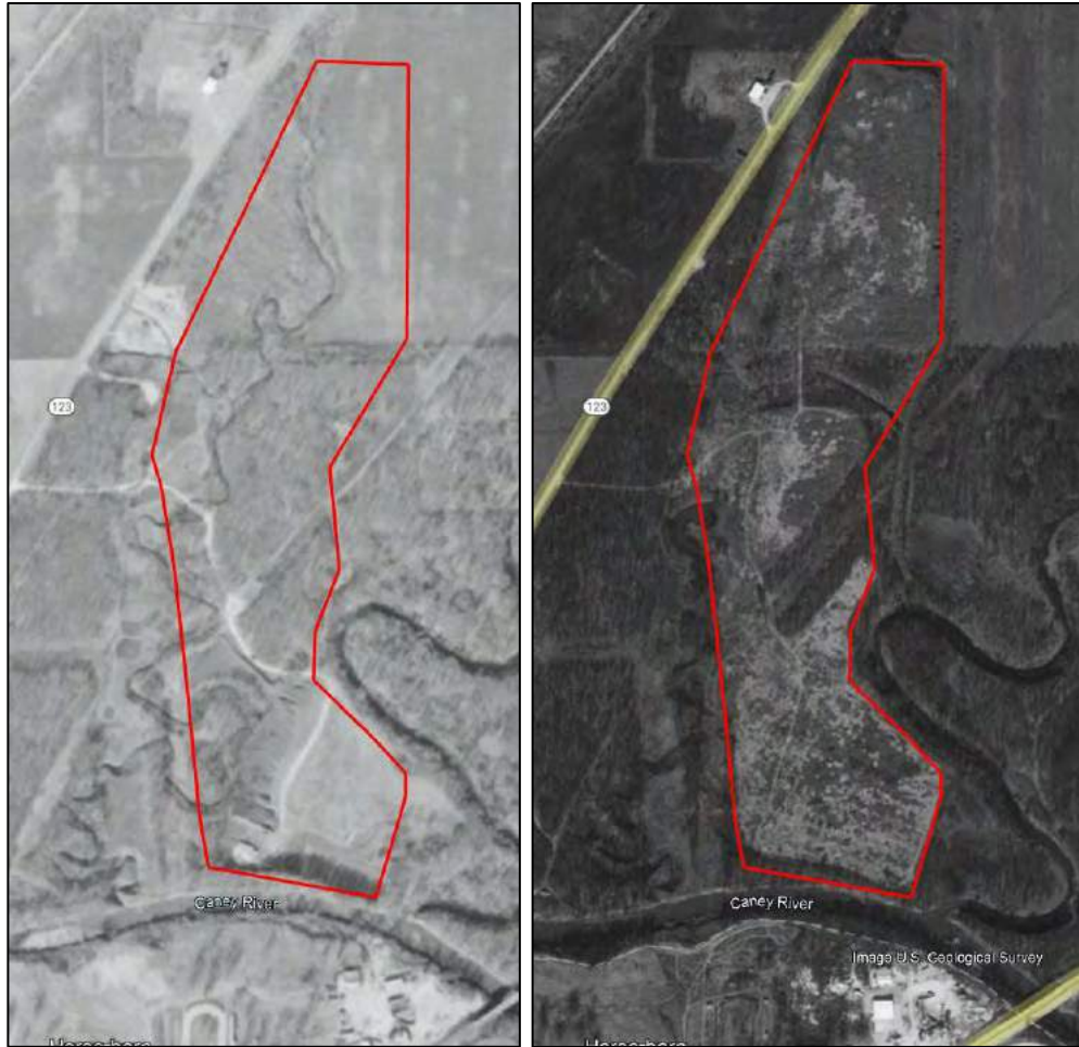
Aerial photographs of WN-138 from 1971 (left) and 1995 (right) showing the extent of the disturbance at those dates. Note the change in the drainage on the west side of the mine and the clear removal of much material from the mining.
