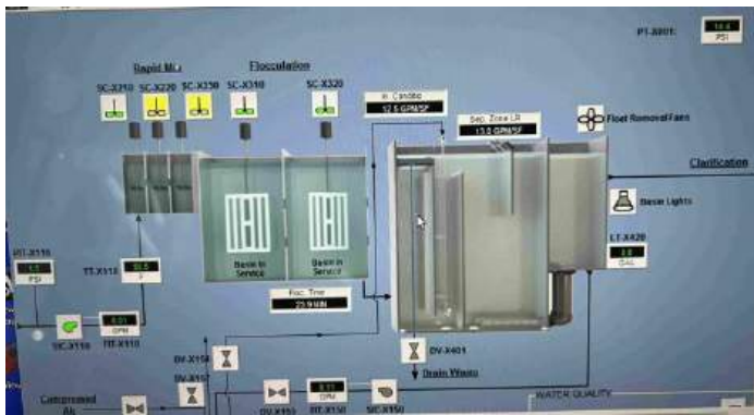
Rapid Mix/Flocculation HMI Screen
