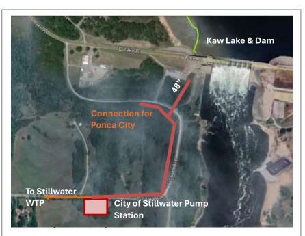
Figure 2-2 Kaw Lake Intake Pipe for Stillwater and Ponca City
