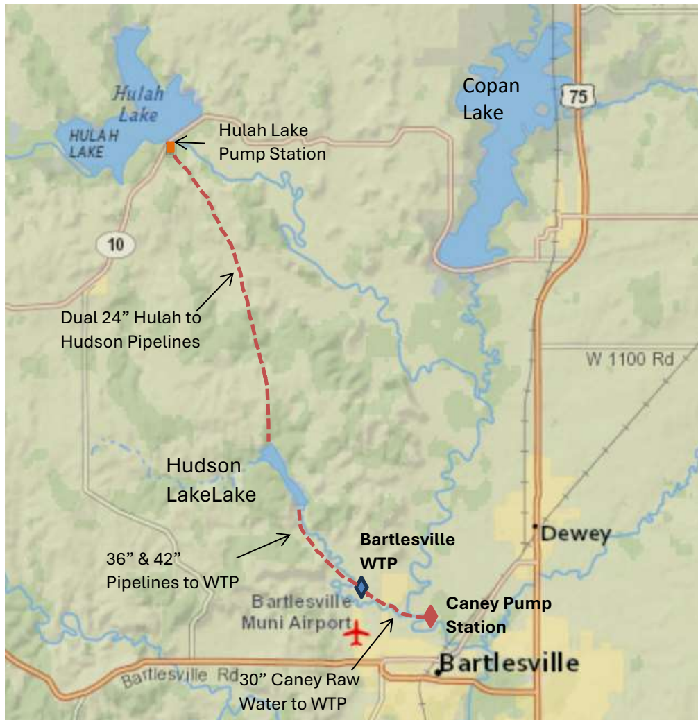
Figure 1-9 Bartlesville's Existing Water Supply
