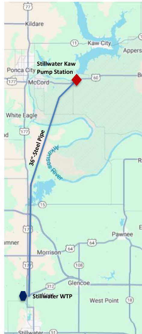
Figure 1-5 Stillwater Raw Water Conveyance System
