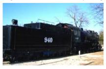
but it has now been relocated to the City's historic **Santa Fe Depot** at 2<sup>nd</sup> and Keeler. The 900-class/940 series were the first locomotives to burn fuel oil instead of coal and were synonymous with the Santa Fe engine. Built by Vulcain, this Santa Fe engine, built in 1903,
