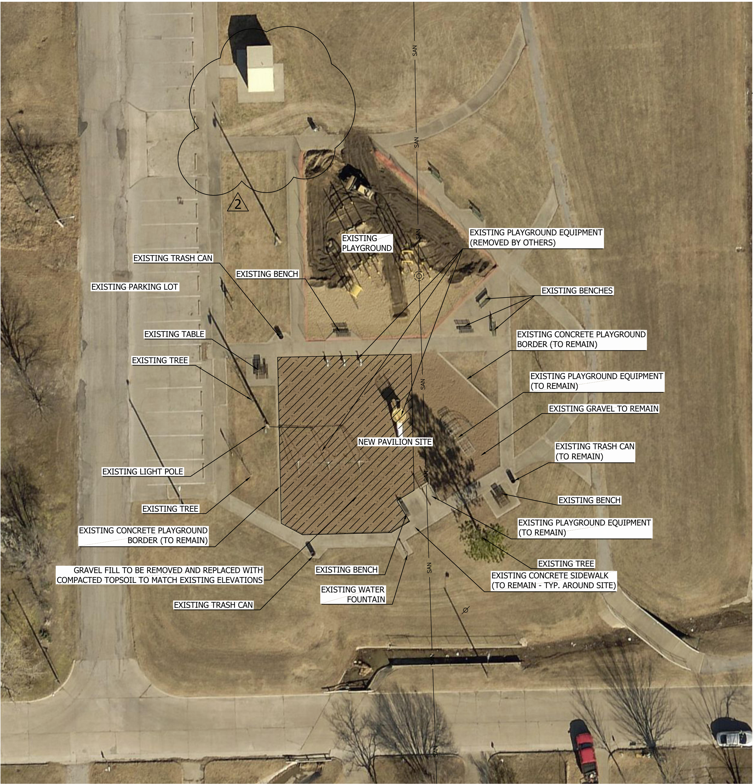
A EXISTING OVERALL SITE LAYOUT AND DEMOLITION 1" = 20'
